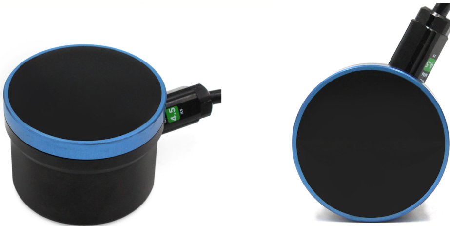
Figura 3.6: Ecosonda Ping Sonar monohaz (Blue Robotics).
