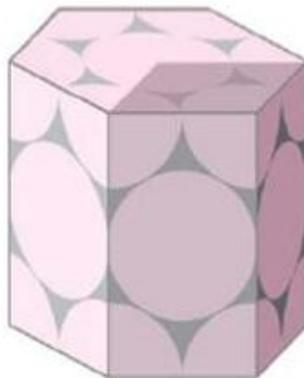
Figura 1.3 Estructura hexagonal compacta HCP
