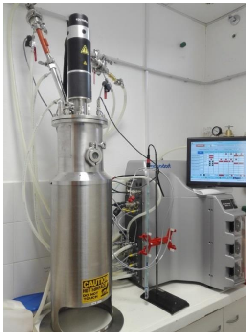
Figura 3.2: Biorreactor New Brunswick™ BIOFLO 415 SIP Fermentor.
